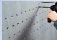
Serial drilling to make 35 holes of \phi 18 \times 70\text{mm} from one full charge.
