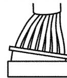
Before connecting the harness, apply grease to the connector terminals. Insert the switch connector all the way, making sure that there is no gap between the connectors.
