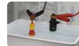
(Image photo) Input 10,000VAC for 3 minutes with insulated manual grip by immersing in water pool.
