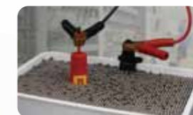
(Image photo) Input 10,000VAC for 3 minutes by immersing in metal ball pool.
